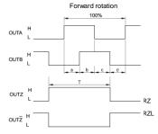
Forward rotation means clockwise revolution viewed from the shaft. 12.5%≤a,b,c,d≤37.5%, 50%≤T≤150%
